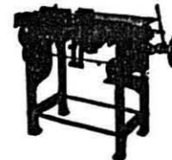
PETERS JUNIOR CARTON FOLDING AND CLOSING MACHINE (right) closes 35-40 cartons per min., no operator.
